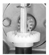
Adjuster drive gear engaged at bottom
