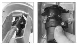
Removing the adjuster from the front
